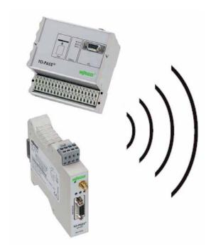
The TO-PASS® product family is designed for wireless communication of signals and messages. Connection is established via the GSM global mobile radio network. Beyond other communication channels (e.g., email, SMS or fax), the devices can also transmit data to a Web server via Web functionality. This allows the creation of a permanent GPRS connection that's similar to a dedicated line.
